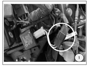
**35** IND and Europe: Connect flasher's extension Negative terminal cable with battery as shown. Ensure proper cable routing as shown.
