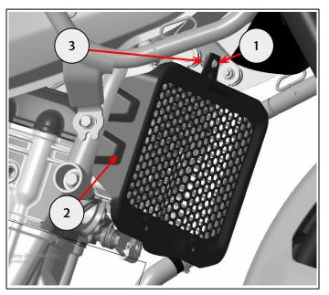
**3** Place a spacer from the kit (1) between the radiator guard (2) and the motorcycle's mount point (3). Fit fixing M6 x 35mm (4) through the radiator and spacer. Do not fully tighten at this stage. Repeat for the remaining spacer and fixing.
