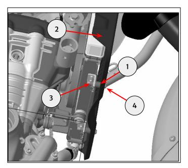
**4** Tighten the lower fixings (1) to **10Nm**. Tighten the top fixing (2) to **10Nm**.
