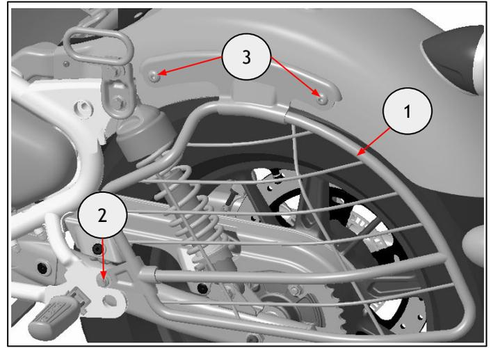
**5** Remove the fixings (1) on the right side of the mudguard.
