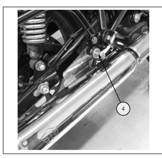
**9** Ensure the clamp is in the correct orientation as shown and positioned correctly over the inlet pipe of the silencer. Tighten the clamp to *30Nm*.
