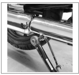
**10** Tighten the rear mount fastener (4) to **25Nm**.
