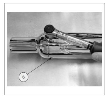
**6** Insert the new gasket (3) from the kit into the accessory silencer (1) inlet, ensuring none of the gasket is protruding. Position the existing clamp over the inlet as shown.
