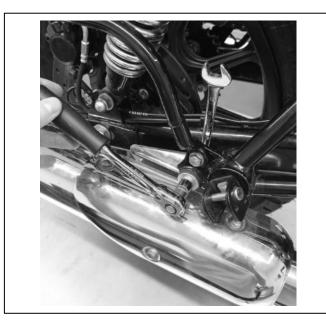
**3** Slide the silencer assembly from the end of the exhaust pipe.
