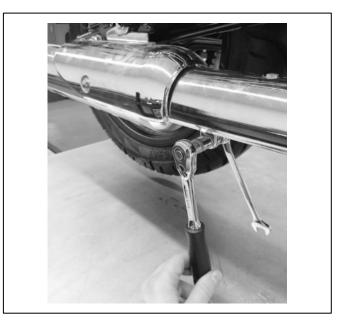
${\bf 2}$  Remove the silencer mount bolt and nut. Discard the bolt and retain the nut.
