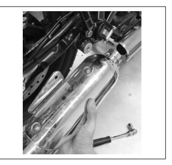
**4** Remove the silencer mount bracket by removing 2 M8 bolts. Discard the bolts. Retain the bracket for fitment to the accessory silencer.
