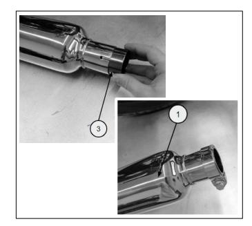
**7** Assemble the existing bracket to the rear of the accessory silencer using 2 M8 bolts (5) from the kit. Ensure the bracket is in the correct orientation as shown. Tighten the bolts to 25Nm.
