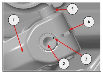
**3** Position the toe piece (1) to the desired position within the adjustment range. Tighten the fixing (2) to **8Nm**.
