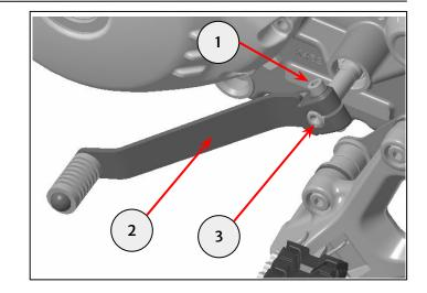
**2** Fit the new gear lever (1) to the splined shaft (2), lining up the shaft mark (3) to the top of the gap in the lever (4). Refit the fixing (5) and tighten to **10Nm**.
