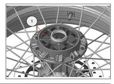
**9** Push the sprocket assembly (1) from the kit into the cush rubbers (2).
