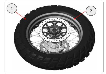
**7** Fit the tyre (1) on the new wheel (2). The tyre rotation arrow should be pointing forward.
