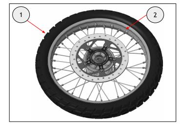
**3** Fit the tyre (1) on the new wheel (2). The tyre rotation arrow should be pointing forward.
