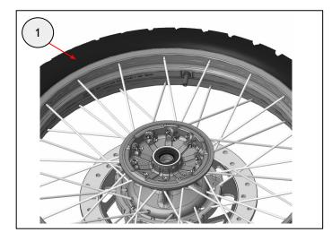
**4** Reassemble the front wheel as described in the Owner's manual.
