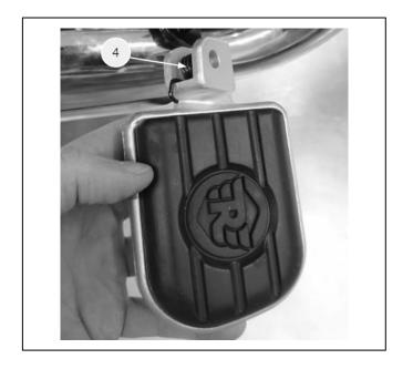
**5** Position the deluxe footpeg (5) inside the clevis on the vehicle and insert the clevis pin (2), ensuring this passes through the center of the spring.
