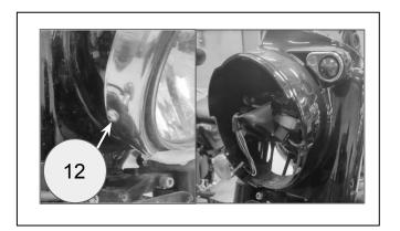
BSVI Meteor: Remove headlamp screw 2Nos (13) and remove headlamp from headlamp assy by removing headlamp connector. retain screw (13) for reuse.
