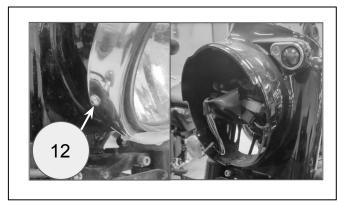
BSVI Meteor: Mount the headlamp to headlamp assy and reuse screw (13) 2 Nos, torque the screw (13) to 5Nm.
