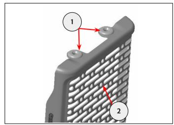
**7** Locate the top of the new oil cooler guard (1) onto the oil cooler locating pins (2) and push downwards. Using the fixings from the kit and the nuts removed in step 4 (3), secure the oil cooler and new cooler guard to the bottom mounts. Tighten to **10Nm**.
