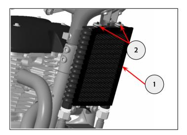
**4** Remove the two fixings (1) and nuts (2). Note: some models are fitted with a fixed plate where the nuts will remain in place.
