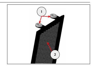
**6** Refit the grommets (1) to the new oil cooler guard (2).
