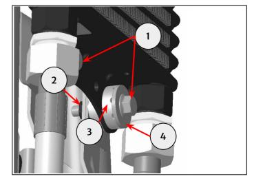
**5** Remove the grommets (1) from the standard oil cooler guard (2).
