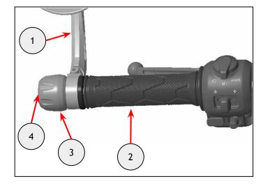
**5** Adjust and set the mirror (1) to a comfortable viewing position. Tighten the fixing (2) to **8Nm**.
