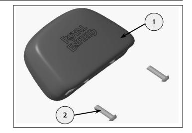
**6** Use the passenger backrest pad retained from step 5, place it over the grab rails, use fixings (2) retained from step 5 to mount as shown. Tighten to **25 Nm.**
