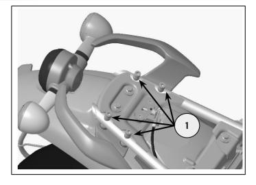
**2** Remove Saree guard mounting fixing (1) from the Left hand side of motorcycle and discard. Remove the existing grab rail .
