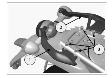
**4** Use fixing (3) from the kit to mount Saree guard mounting bracket(2) with grab rail right hand (1) as shown. Tighten to **10Nm.** Assemble back the seat removed in step 1.
